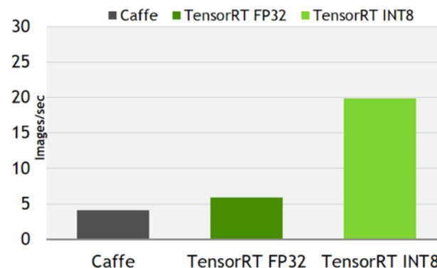
Batch Size = 1, Input/Output Resolution = 512 x 1024
